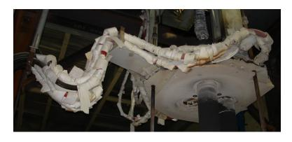
radiant heat and occasional flame impingement. Historically the company has installed high temperature ceramic tape to protect these lines. However, due to the dynamic nature of this application the ceramic tape quickly breaks down and loses coverage (see photo above) and the lines are once again vulnerable to extreme temperatures.
